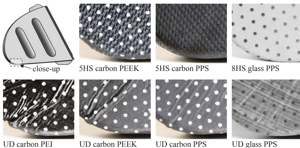
Figure 4.1 Close-up view of press-formed CFRTP stiffening ribs with different materials.
