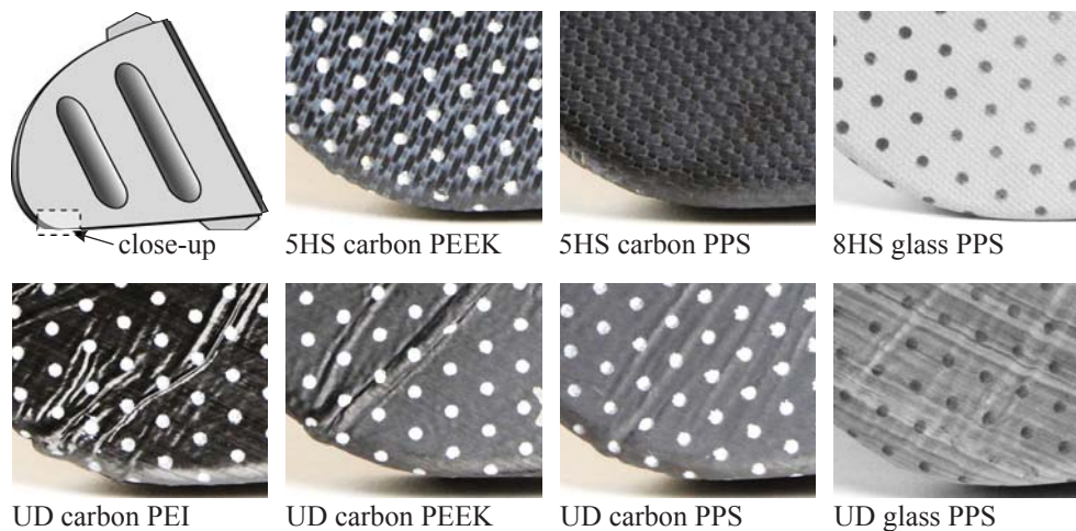
Figure 1.3 Quasi-isotropic CFRP laminates of different materials pressed to stiffening ribs suffer from different severity of formability problems (Chapter 3).
